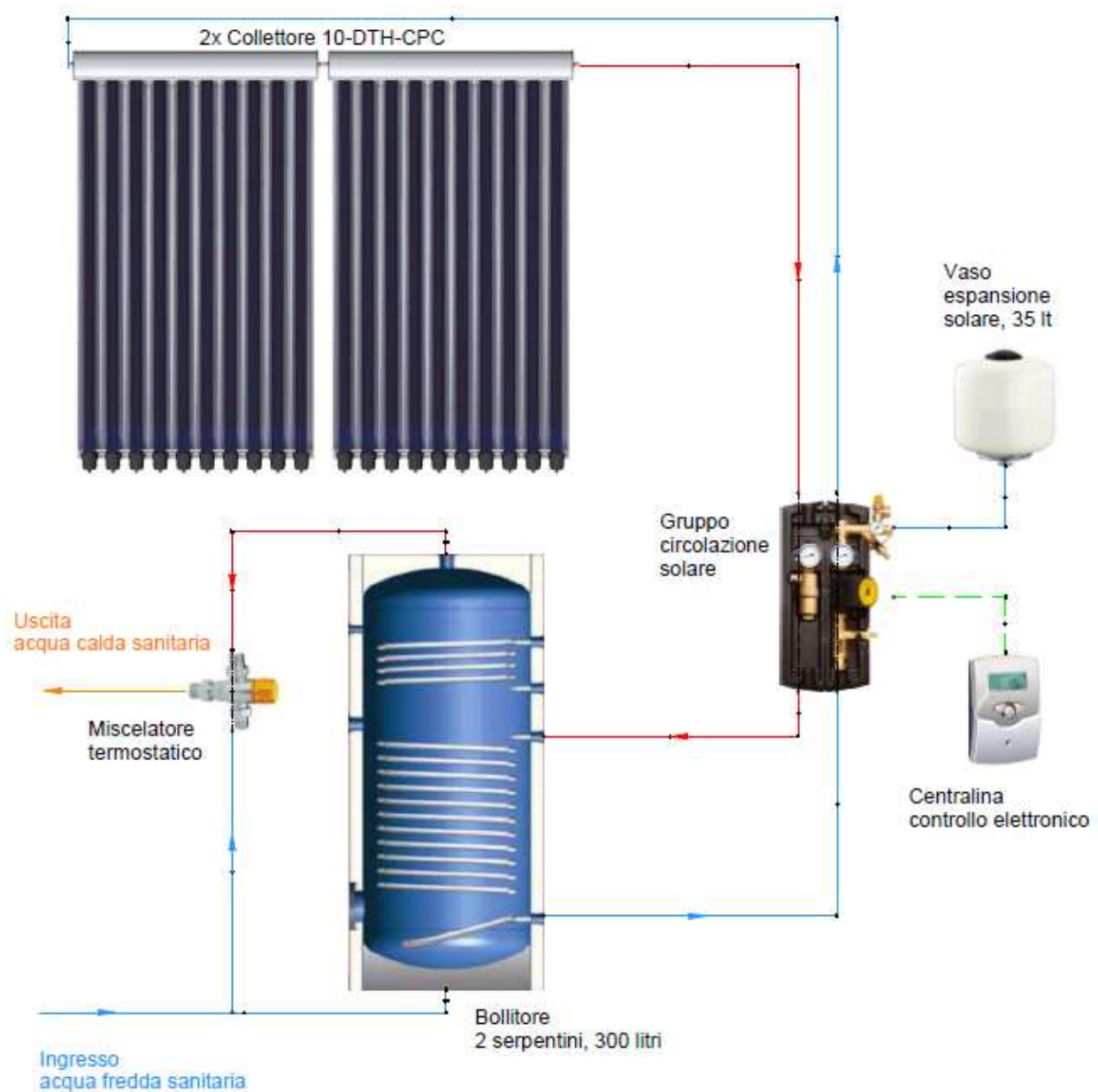
Hot sanitary water solar plant: 2x 10 DTH-CPC collectors and 1 x tanks with 300 litres
